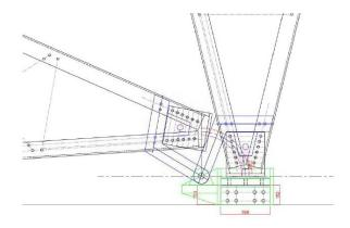
Figure 6: One of the Swivel Base Adapter Proposed Designs
